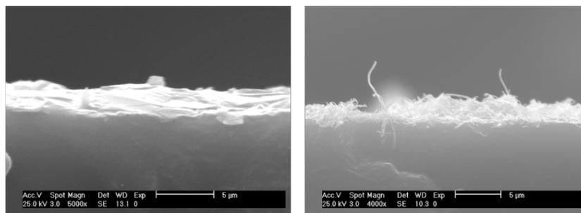
Fig 2. Graphite (left) and Carbon Nanotubes (right) as compliant electrodes
