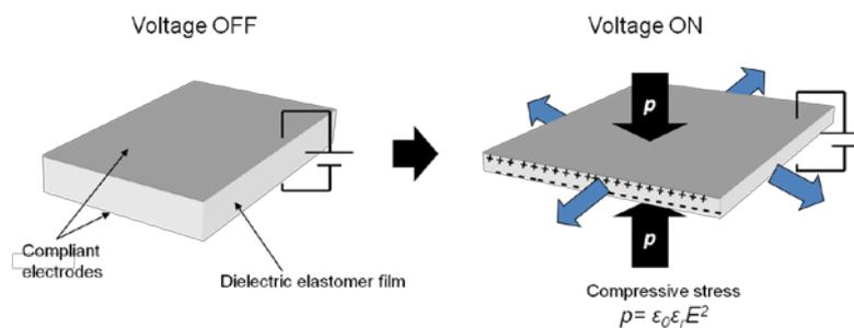
Fig 1. Schematical view of DEA operating principle
